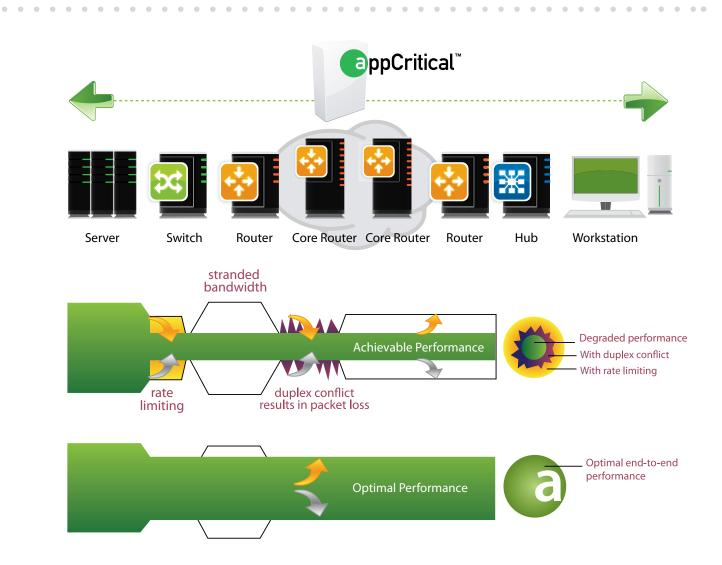
AppCritical focuses on the network paths used by application traffic. With its unique, lengthwise view, AppCritical provides visibility into performance problems anywhere in your network infrastructure, even in parts of the network you do not own — such as your service provider's cloud. It gives you a more effective way to assess, measure and diagnose converged networks.
